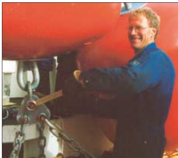
Assembling of shackle to connection plate.
